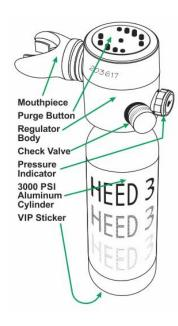
**Regulator Body** - Our simple rugged design utilizes the same time proven technology found in typical regulators used by SCUBA Divers around the world. Our always-on, breathe on demand, balanced single stage regulator is easy to use, maintain and service. HEED 3 can be used in any orientation, even upside down. **Pressure Indicator** - Dial Gauge has an easy to read, color coated display for ataglance pressure check in psi and bar.
